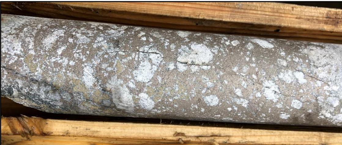
Photo 1 – LPDD19-001 – 140.5m – Semi-Massive Sulphide in Brecciated Gabbro
