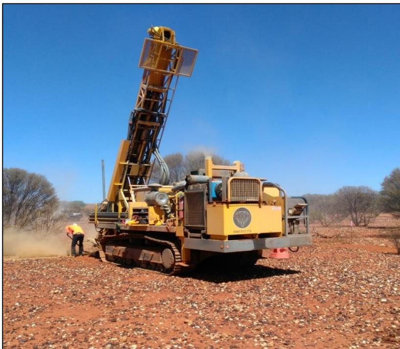
**Image 1** – Track mounted multi-purpose aircore/RC drill rig working at the White Rose Prospect, Munarra Gully Project
